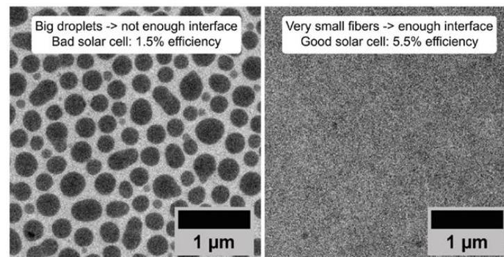
Figure 2 - Top view microscopic image of a bad solar cell (left) and a good solar cell (right), taken with an electron microscope.
