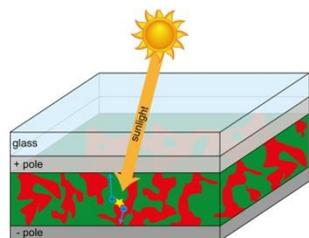
Figure 1 - Diagram of a plastic solar cell.
