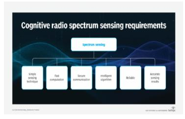
Cognitive radio devices track spectrum bands using a technique called spectrum sensing, which comes in two flavors (cooperative and non-cooperative) and has certain requirements.
